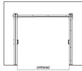
The stacked doors will not hang over into the opening in the fully opened position, with a minimum wall overlap of 5" on each side.
