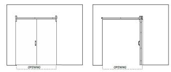
The stacked doors will hang over into the opening up to 4" in the fully opened position, with a minimum wall overlap of 1" on each side when fully closed.
