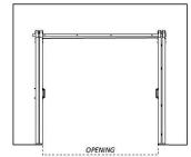
The stacked doors will not hang over into the opening in the fully opened position, with a minimum wall overlap of 5" on each side.
